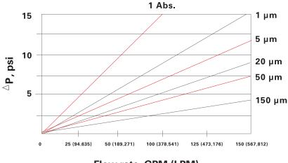
Flow rate, GPM (LPM)
