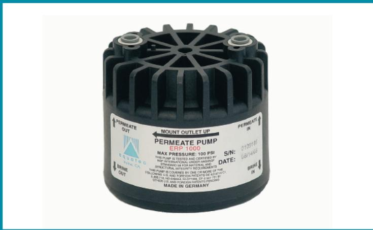
Aquatec's original Permeate Pump (ERP1000) is a simple, yet revolutionary, device. Powered only by the hydraulic energy of brine water usually lost to the drain (i.e. no electricity required), the Permeate Pump forces product water into the storage tank, reducing membrane back pressure and maximizing available feed pressure. These pumps dramatically improve the efficiency of R.O. water production, reducing wastewater by up to 80%. In other words, if your current system requires 10 gallons of tap
